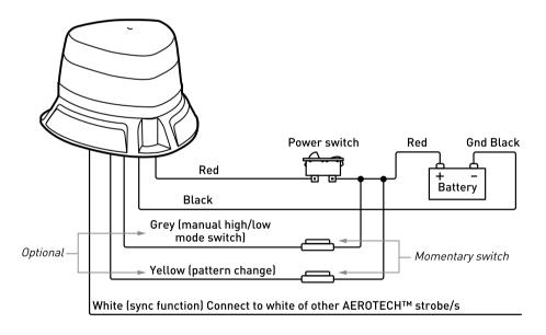
**Note:** To ensure that the light sensor works correctly don't cover the top of the strobe otherwise the senor will register as night mode. Then you will need to connect the override wire (Grey) to a momentary switch to allow them to switch to "High/Low power mode".
